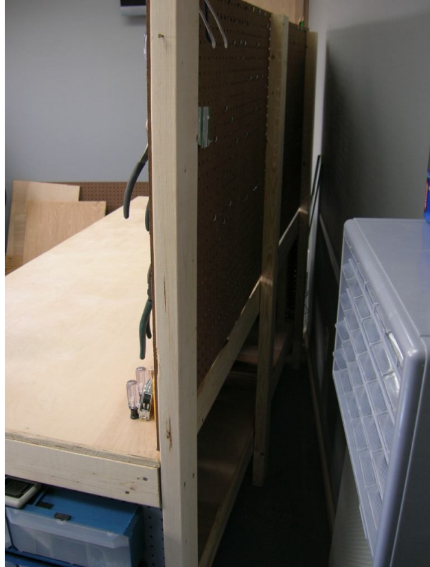
Photo 4 - Pegboard Back Bracing
